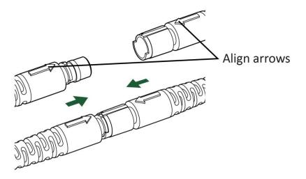
3. Place CableLok Top over connectors align ridge with corresponding ridge on connector
