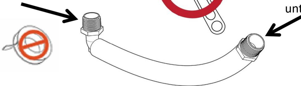
\*Use of Teflon tape inside Irrigreen sprinkler heads or not mounting Irrigreen sprinkler heads on Flex-Pipe voids the sprinkler warranty.
