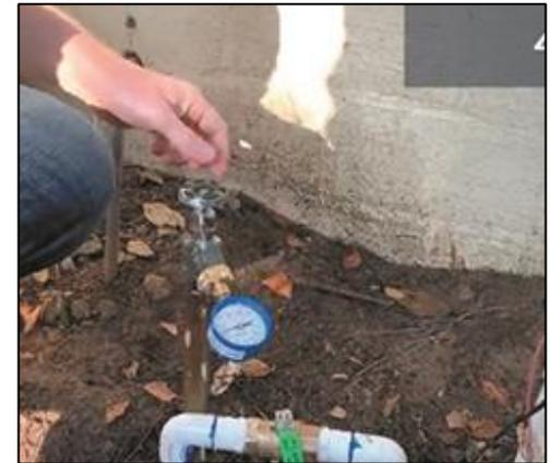
**Connect a pressure gauge to the water spigot to check pressure.**
